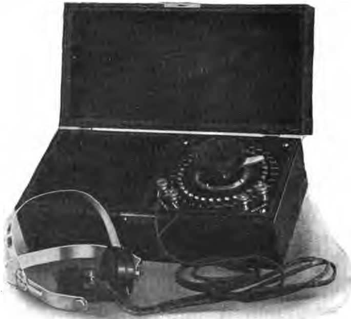
Fig. 238—Audibility Meter (American Marconi Company).
